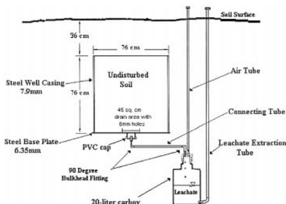
**Figure 2.** Lysimeter used to collect percolated water and leachate under plots in each treatment in the Rodale Farming Systems Trial.
